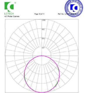
Maximum Candela = 1308.84 Located At Horizontal Angle = 0, Vertical Angle = 0 # 1 - Vertical Plane Through Horizontal Angles (0 - 180) # 2 - Vertical Plane Inrough Horizontal Angles (WU - 270)
